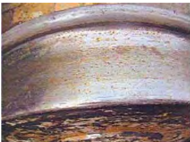
Figure 6: Circumferential cracking associated with rollover
